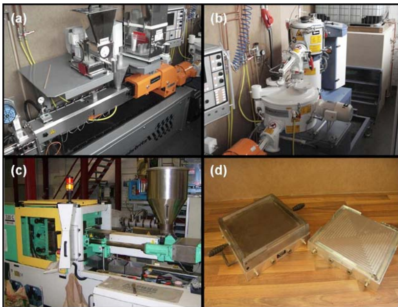
Figure 1: Various processing technologies for WPC production (a) Twin screw extruder, (b) hot cool mixer unit, (c) injection moulder, (d) compression moulding die
