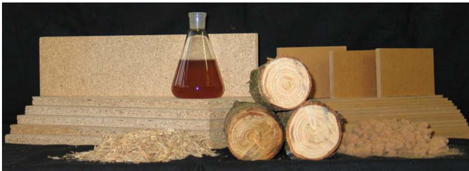
Figure 10: Wood of low quality might be used to produce particles or fibres that subsequently might be pressed into particle boards (shown at the left) or MDF (medium dense fibreboards shown at the right). Kharazipour and colleagues developed processes in which fungal laccases from cultural supernatants (the brown liquid seen in the flask) are applied in glueing particles or fibres in order to replace chemical binders made from non-sustainable crude oil (further information in Kües et al. 2007a).
