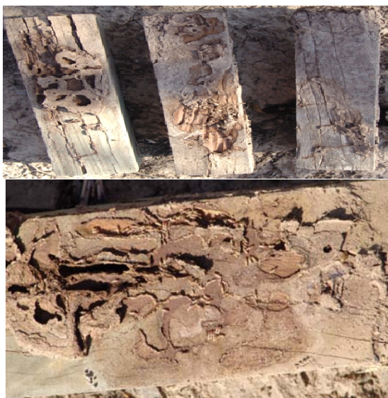
Fig 8-Control samples of E. camaldulensis in Albaji and Mishmast station, the attack by termites started after 36 month and then the grade No. reached to 6.7 after 118 month
