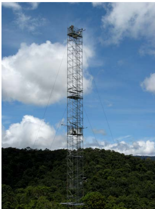
Fig. 1: The main measurement tower at the site in Bariri rainforest (height: 70m):
