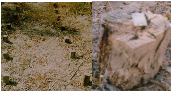
Fig. 19- Treated with Creosote samples are sound and Control samples are attacked
