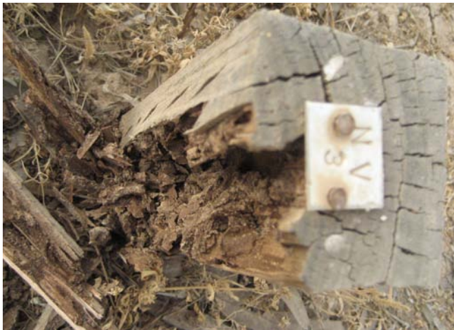
Fig 15- Control samples of E. viminalis in Albaji, the attack by termites, and grade No. reached to 0 after 24 month
