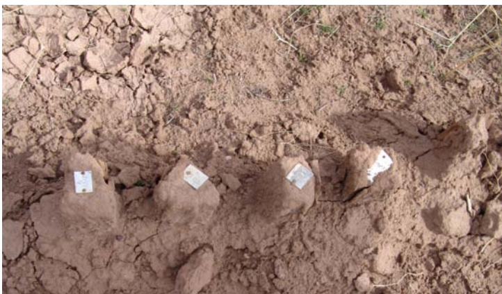
Fig 18-Samples are covered with mud by termites for protecting them against sunlight
