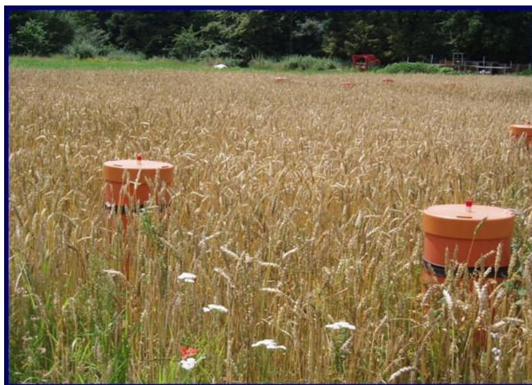
Fig. 2: Closed chambers for gas sampling in a wheat field in Darmstadt, Germany in July 2007
