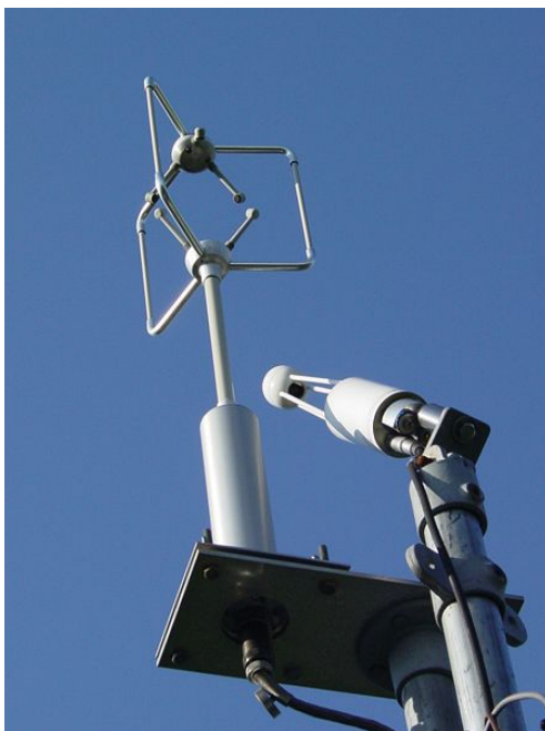
Fig. 2: Ultrasonic anemometer (Campbell CSAT3, left) and infrared gas analyzer (Li-Cor 7500, right) (Burba, 2007).
