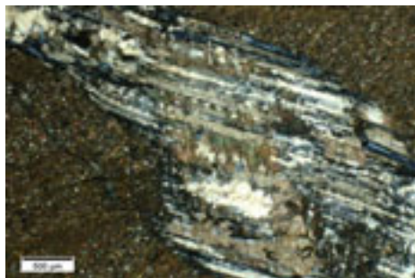
Figure 2: This vein gives an example of a vein on which the ‘crack seal’ models given so far can be critically tested on. How did the various minerals quartz, chlorite and calcite get deposited in one vein? Sample from 1392.5 m TVD.
