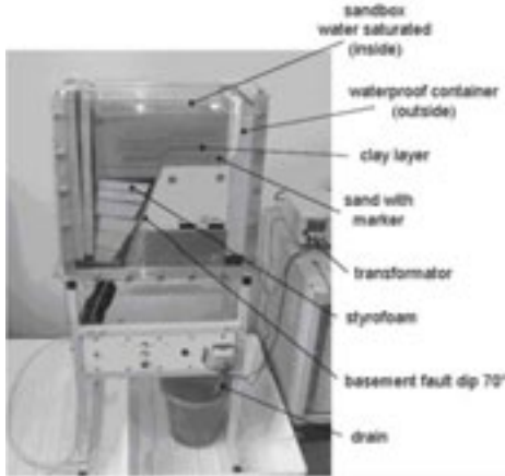
Figure 1: Sandbox-apparatus. Water-saturated setup of layered sand-clay experiment. Stage: Immediately after deformation.
