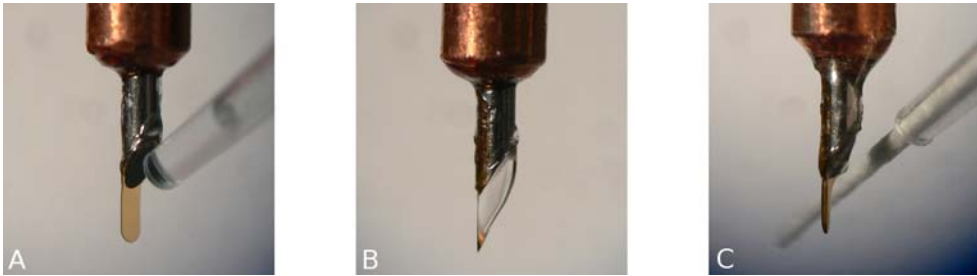
Figure 4.18: Application of cell suspension to sample support. (A) A small volume of cell suspension (between 1 and 2\ \mu\text{l} ) is placed onto one side of the hydrophilized polyimide foil. (B) Ideal wetting result after application of the droplet. (C) Removal of excess liquid using a paper wick immediately before the sample is injected into liquid ethane. Figure adapted from [56].
