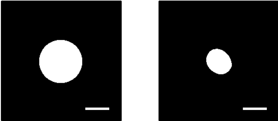
Figure 6.7: (Left) Initial binary mask applied to the illumination function, back propagated to the aperture plane. (Right) Final mask as obtained after several iterations of the Shrink-Wrap procedure, see main text. The scale bars indicate 2 \mu\text{m} .
