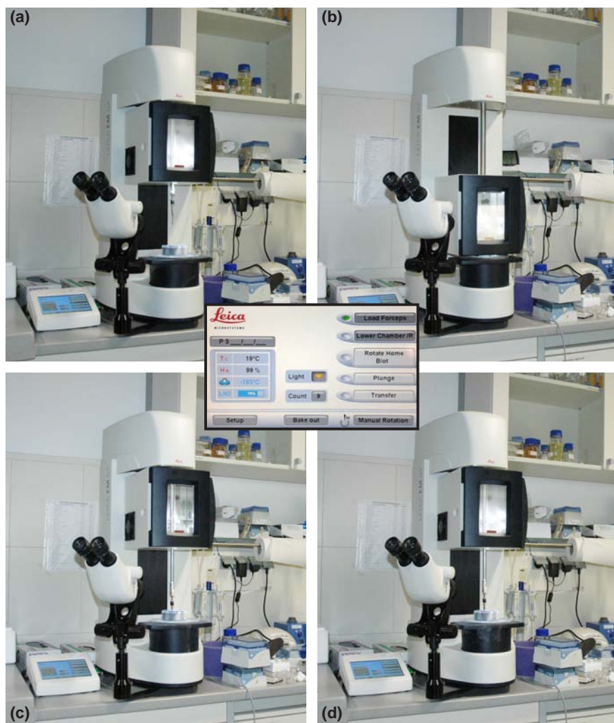
Fig. 4.2: Photographs of the grid plunger in the different positions during plunge-freezing. (a) Load Forceps position, in which the sample can be attached to the plunging rod and the chamber is moved upwards. The inset shows the display of the controlling software. (b) Lower Chamber position, in which chamber is moved downwards and the sample is blotted. (c) Plunge position, in which the sample is plunged into the ethane bath and afterwards the chamber is moved upwards. (d) Transfer position, in which the sample is slightly lifted in the ethane bath allowing for the transfer to a cryovial.
