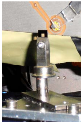
Fig. 5.1: \text{Si}_3\text{N}_4 membrane window mounted on a crocodile sample holder (ID13, Nov. 2011).
