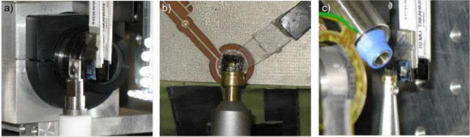
Figure B.4: a) Hydrated sample at the P10 beamline (DESY), the beam is coming from the right and travels towards the left. b) Freeze-dried sample at the ID13 beamline (ESRF), the beam is coming from the back and travels towards the eyes of the reader. c) Cryoprotected sample at the P10 beamline (DESY), the cooling system is represented by the blue part, the beam direction is the same as in a).
