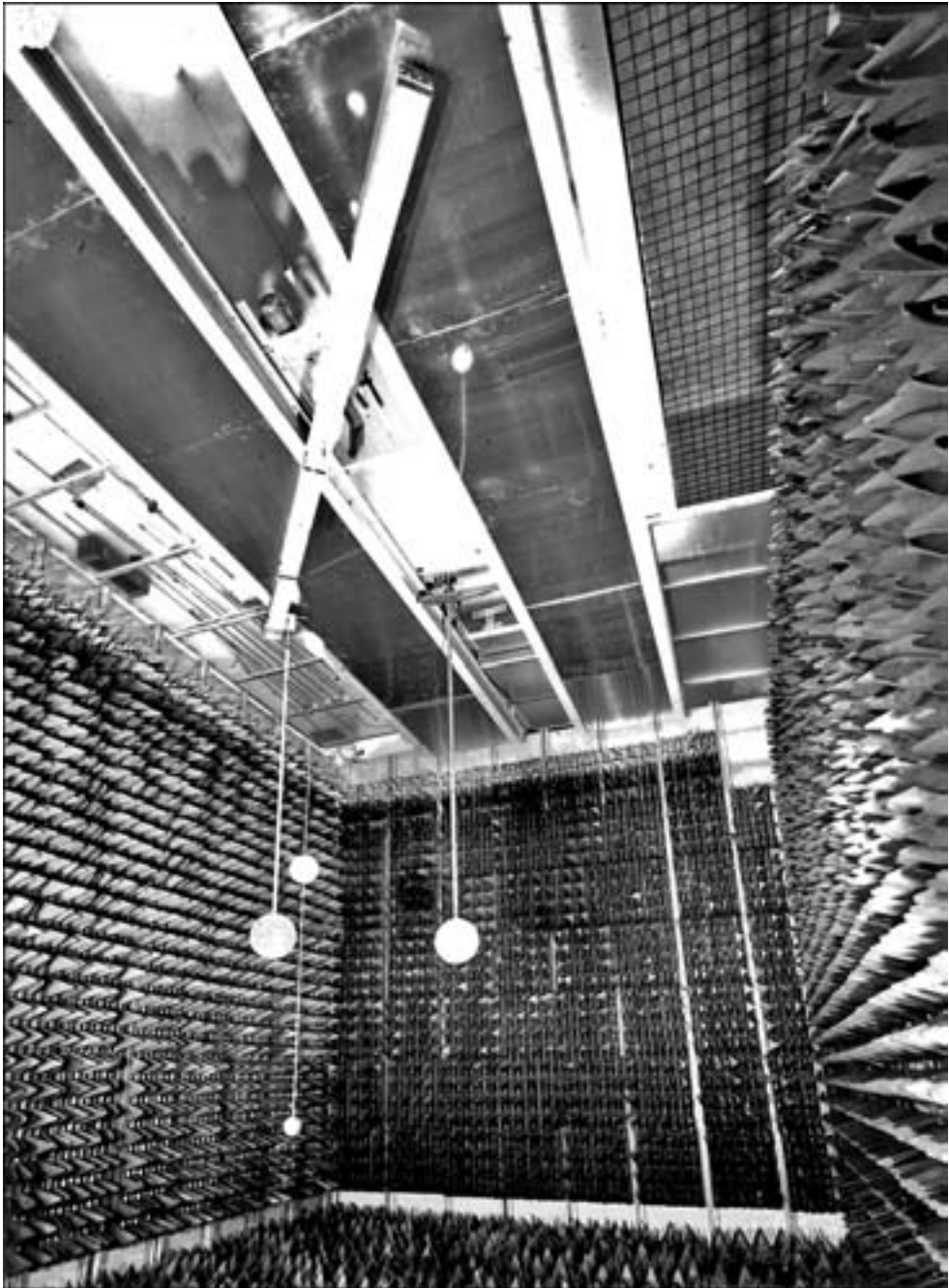
Anechoic water tank lined with rip-type absorbers.
