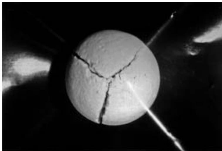
Figure 13. First cleavage of a 15 mm diameter stone as in Fig. 12 but in three cleavage surfaces. The positive pulse pressure amplitude was 37 MPa in the experiment. The direction of wave propagation was perpendicular to the figure plane.
