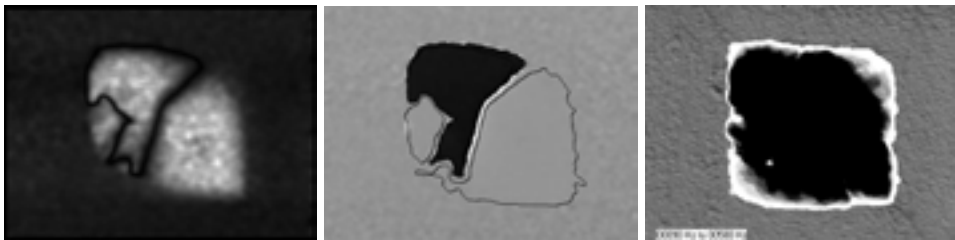
Figure 12. ESPI-study of vibrations of an artificially produced detachment in a plaster layer on a stone wall. Left: amplitude map of 230-Hz higher-order mode of the plaster plate; centre: corresponding phase map; right: final evaluation of excitation response between 90 Hz and 580 Hz in 10 Hz-steps indicating the loose area (dark illustrates frequently, bright rarely excited regions) – an ordinary object image in the background.
