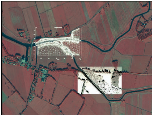
Terrain discretisation and remote-sensing-based roughness determination for a flood simulation
